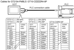
\*1 The cable for GT2104-PMBD does not have the connection to a signal name (RSA, RSB, CSA, CSB).
