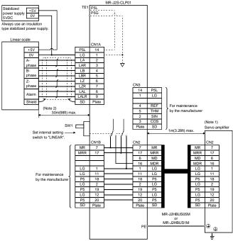
Note 1. For servo amplifier wiring, refer to the servo amplifier specifications guide.
