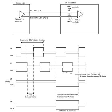
Note: The linear scale that does not include Z-phase is inapplicable.
